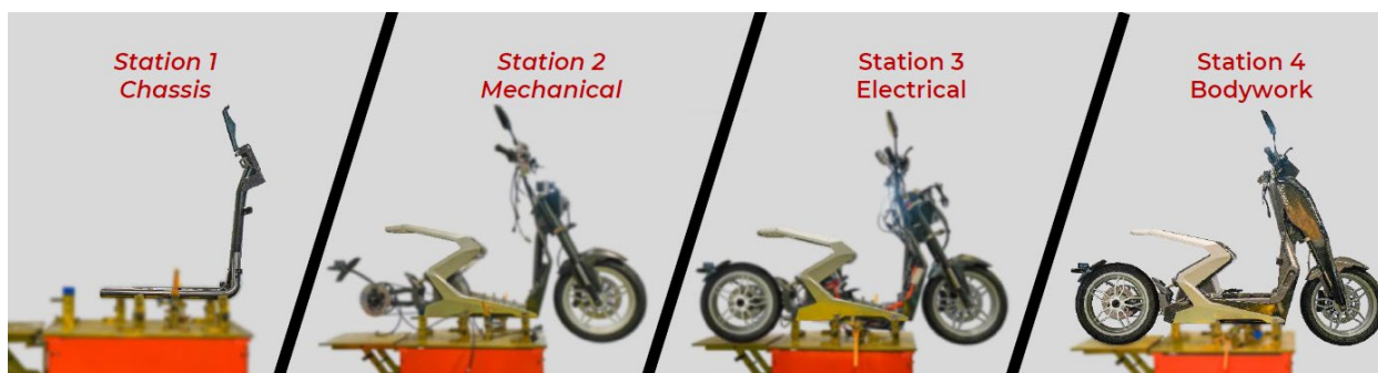
Figure 9 – Zapp Electric Vehicles Group Ltd. – Simplified Assembly
